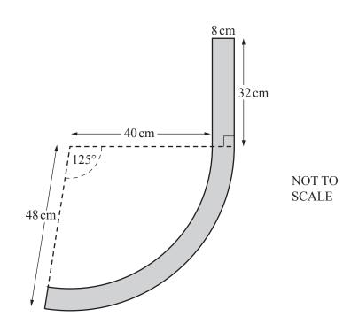
The diagram shows the cross section of part of a park bench. It is made from a rectangle of length 32 cm and width 8 cm and a curved section. The curved section is made from two concentric arcs with sector angle 125°. The inner arc has radius 40 cm and the outer arc has radius 48 cm.
