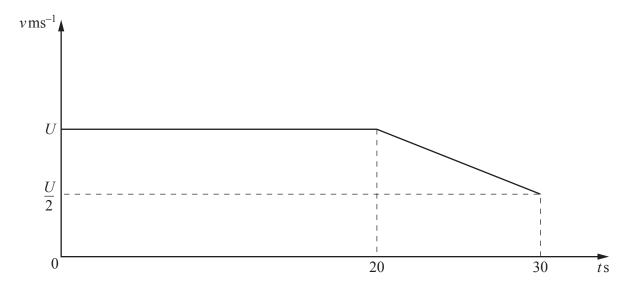
The diagram shows part of the velocity-time graph for a particle, moving at  $v \, \text{ms}^{-1}$  in a straight line,  $t \, \text{s}$  after passing through a fixed point. The particle travels at  $U \, \text{ms}^{-1}$  for 20 s and then decelerates uniformly for 10 s to a velocity of  $\frac{U}{2} \, \text{ms}^{-1}$ . In this 30 s interval, the particle travels 165 m.
