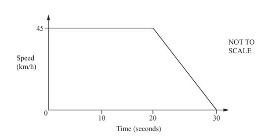
The diagram shows the speed-time graph of a car. The car travels at 45 km/h for 20 seconds. The car then decelerates for 10 seconds until it stops.
