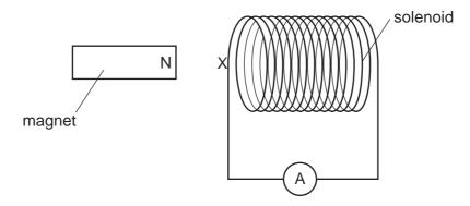
First, the N pole of the magnet is pushed towards X, then the magnet is pulled away from X. During both stages the ammeter deflects.
