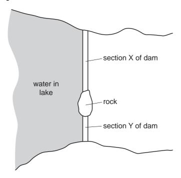
The water creates a total force on each section of the dam and an average pressure on each section of the dam.
