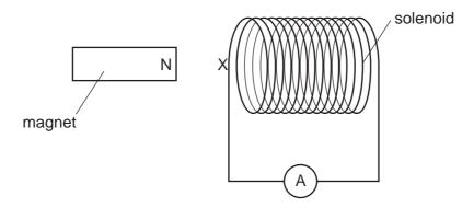
First, the N pole of the magnet is pushed towards X, then the magnet is pulled away from X. During both stages the ammeter deflects.
