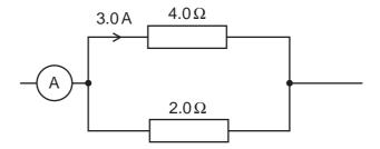
The current in the  $4.0\Omega$  resistor is 3.0 A.
