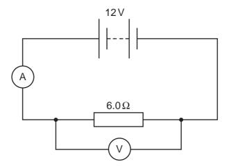
How much energy is transferred by the resistor in 10 seconds?
