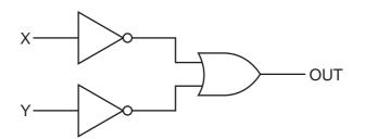
Which single logic gate, placed between X, Y and OUT, would have the same effect as the network?
