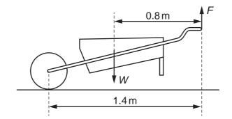
Which vertical force F is needed to support the wheelbarrow in the position shown?
