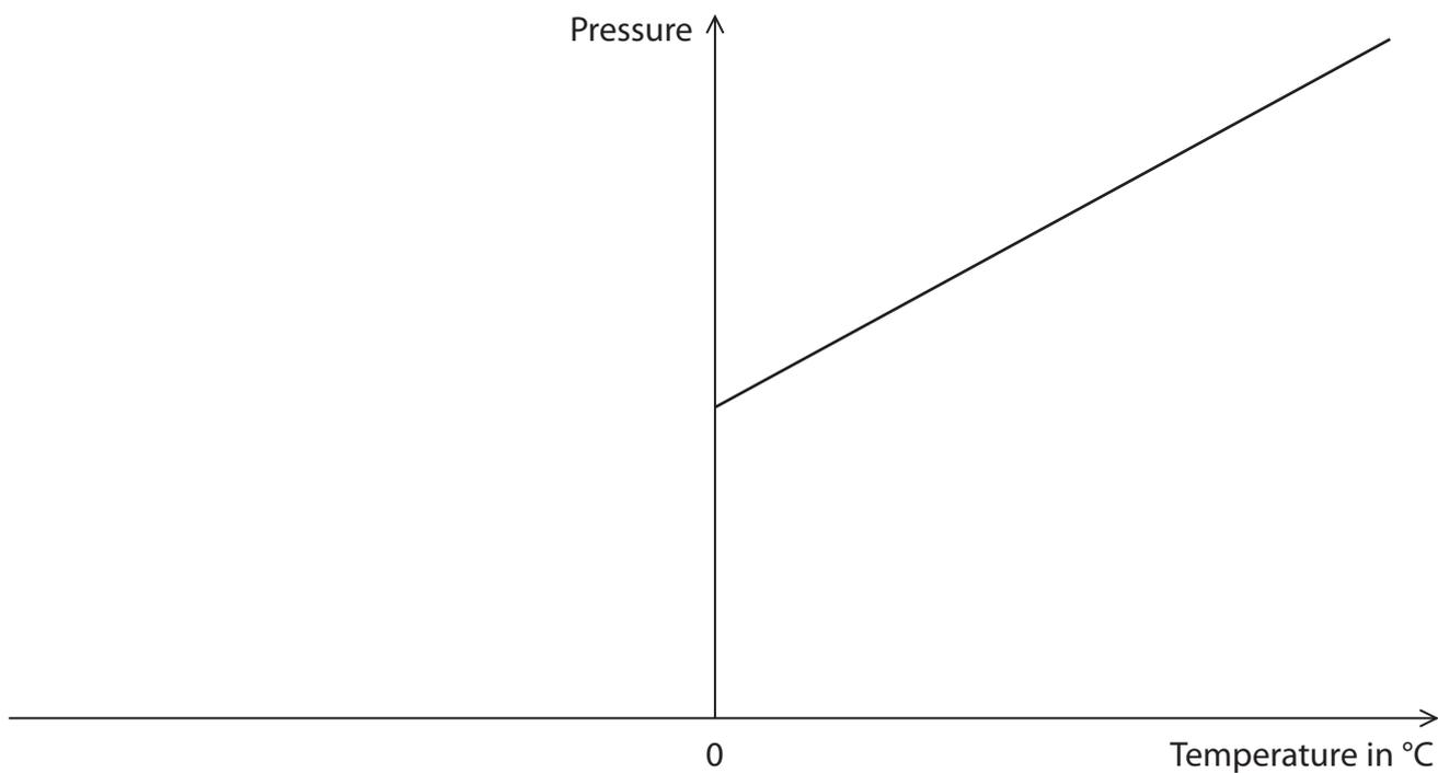
(i) Describe how the graph can be used to show that there is a minimum value of temperature, known as absolute zero.
