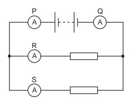
Which two ammeters read the largest current?
