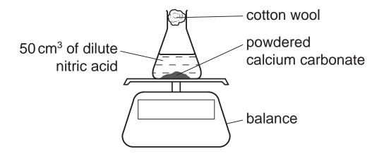
Excess powdered calcium carbonate was added to the nitric acid and the mass of the beaker and contents recorded. The time taken for the mass to decrease by 1 g was measured. The experiment was repeated at different temperatures.
