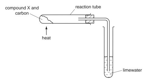
A brown solid is formed in the reaction tube and the limewater turns cloudy.
