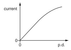
What happens to the resistance of the component in these two sections as the current increases?
