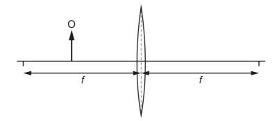
Where is the image formed and how does its size compare to the object?
