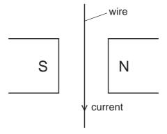
The magnet and current cause a force to act on the wire.
