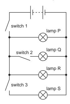
Which switches must be closed to light only lamps P and R?
