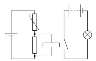
Which change in the environment causes the lamp to be switched on?
