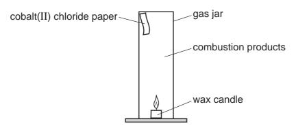
After a short time, the oxygen in the jar is used up and the candle flame goes out.
