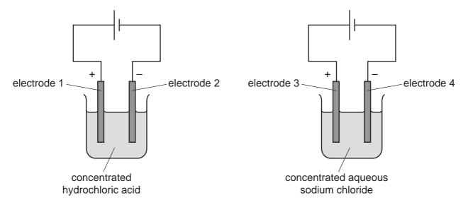
At which electrodes is hydrogen produced?
