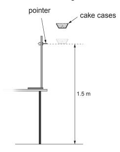
The cake cases are dropped from at least 20 cm above the pointer. This allows them to reach a terminal speed by the time they reach the pointer. The time taken for the cases to fall the distance of 1.5 m between the pointer and the floor is measured.
