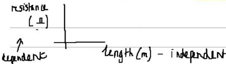
Use a ruler to measure the length of the wire, then use an ammeter to measure the current through the wire and a voltmeter to measure the potential difference across the wire. Use  $R = \frac{V}{I}$  to calculate the resistance for this length.
