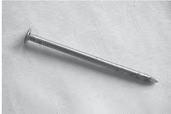
(c) Both ends of the nail exert pressure when the nail goes into the wood.
