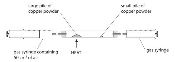
The large pile of copper powder is heated, and the air in the syringe is passed several times from one gas syringe to the other.
