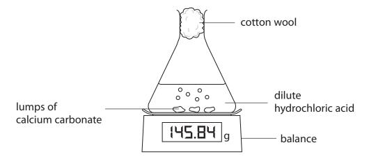
The mass of the flask and contents is measured at regular time intervals.
