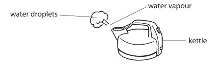
As the water vapour cools it turns into droplets of liquid water.
