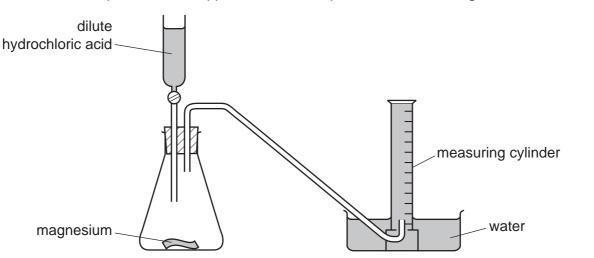
Using a tap funnel, 20 cm<sup>3</sup> of hydrochloric acid was added to 4 cm of magnesium ribbon. The volume of hydrogen produced was measured every minute for six minutes.
