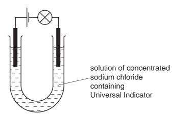
The bulb lit up. The solution near the negative electrode changed colour from green to purple.
