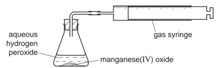
The volume of oxygen released was measured every 20 seconds.
