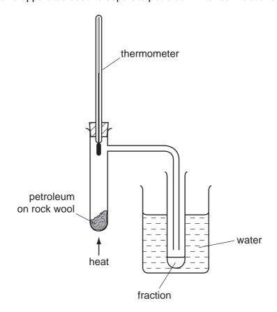
Which fraction contains the smallest hydrocarbon molecules?
