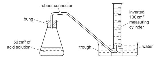
Using a measuring cylinder, 50 cm³ of acid **X** was poured into the conical flask. 0.5 g of magnesium ribbon was added to the conical flask and the bung replaced.
