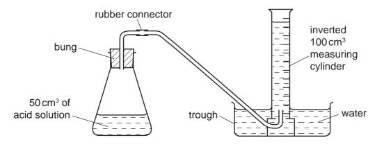
Using a measuring cylinder, 50 cm<sup>3</sup> of acid **X** was poured into the conical flask. 0.5 g of magnesium ribbon was added to the conical flask and the bung replaced.
