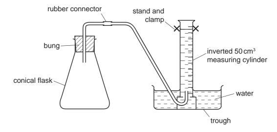
Remove the bung from the conical flask and move the measuring cylinder away from the delivery tube without letting any water run out. Twist one of the strips of magnesium provided to break it into four pieces and place all of them into the conical flask.
