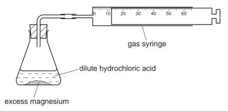
The volume of hydrogen produced was measured every minute for six minutes.
