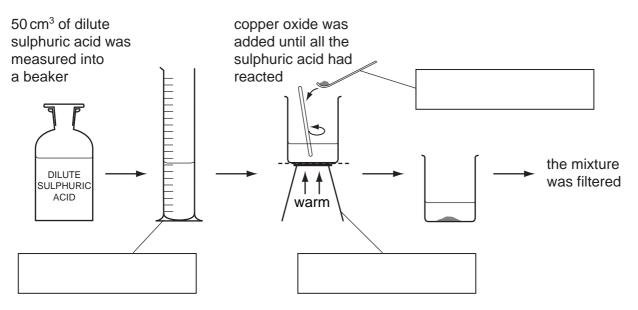
(a) Complete the empty boxes to name the pieces of apparatus.
